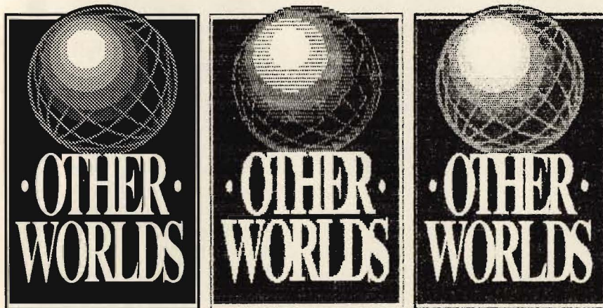
The original 300-dpi PostScript LaserWriter output (left) is closely matched by the 36-dpi Star NX-1000 (center) and 180-dpi Hewlett-Packard PaintJet (right) versions.
